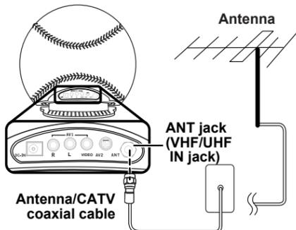
1. Connect one end of the VHF/UHF (Antenna) or CATV cable to ANT Jack (VHF/UHF IN Jack) on the back of the TV.
