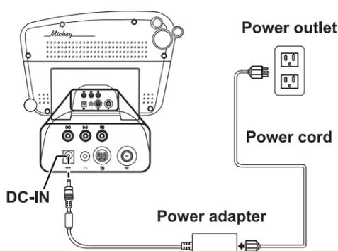
1. Connect the power cord to the power adapter as illustrated.
