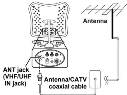
1. Connect one end of the VHF/UHF (Antenna) or CATV cable to ANT Jack (VHF/UHF IN Jack) on the back of the TV.
