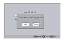
During auto search, the scale value on the progress bar is continually increasing, indicating the auto search is in progress. After finishing the auto search, the TV will play the channel starting the auto search. To stop the search in halfway, just press **Cancle**, and the TV will play the first searched channel.
