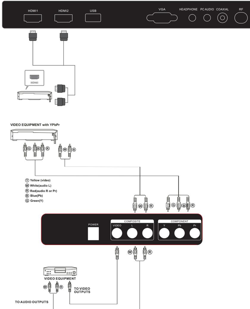
The television's inputs can be connected to the following types of equipment: VCR, multi disc player, DVD, camcorder, video game or stereo system, etc.....
