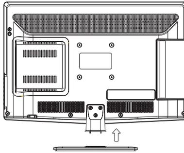
2. Attach the stand base plate to the stand pole by firmly tightening the supplied screw.
