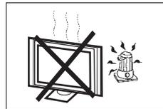
Avoid exposing the television receiver to direct sunlight and other sources of heat. Do not stand the television receiver directly on other products which give off heat, e.g. video cassette players and audio amplifiers. Do not place naked flame sources, such as lighted candles on or near the television.
