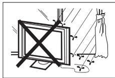
To prevent fire or electrical shock hazard, do not expose the television receiver to rain or moisture.
