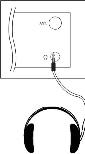
Plug a set of headphones into the 3.5mm mini-jack socket on the rear panel of the set.
