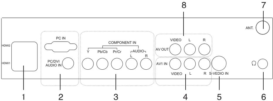
**1 HDMI Input:** Connect a signal to HDMI
