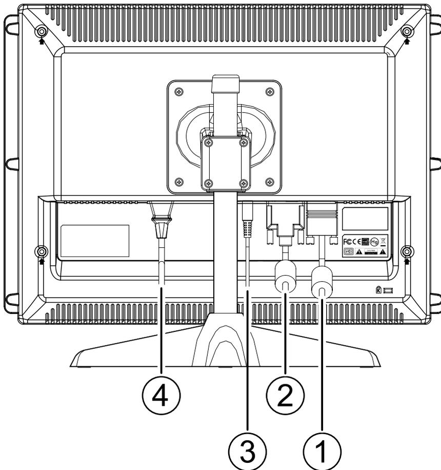
Figure.2. Connecting Cables
