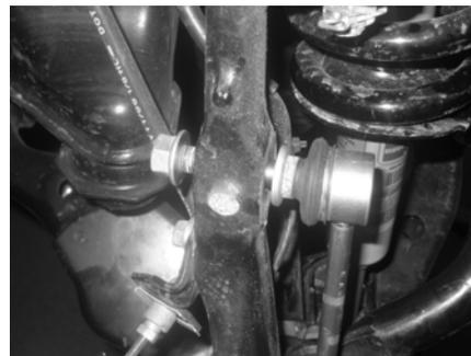
2. Using a 17mm ratchet, remove the nut from the bolt connecting the front sway bar link and the steering knuckle on both sides of the vehicle. HINT: If the ball joint turns together with the nut, use a 6 mm hex wrench to hold the stud.
