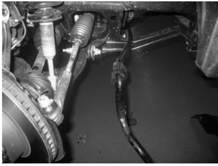
6. Using a 19 mm ratchet, remove the lower two ball joint bolts.
