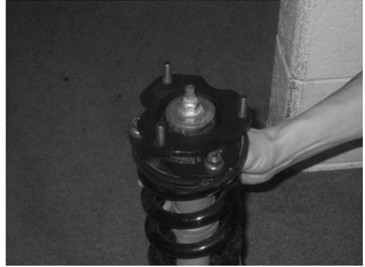
11. Place strut back into upper strut mount. Tighten provided nuts snug with wrench or ratchet (after install, you will torque to OEM specs).
