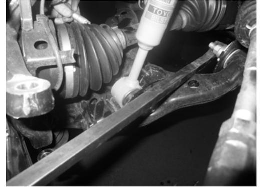
13. Place a jack under the lower control arm. Raise the lower control arm to reattach the lower ball joint bolts. Torque the ball joint nuts to OEM specs.
