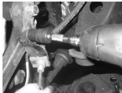
4. Detach all brake hose brackets from the steering knuckle and upper control arm. On vehicles with ABS, remove the front wheel speed sensor-retaining bolt and detach the sensor from the steering knuckle.
