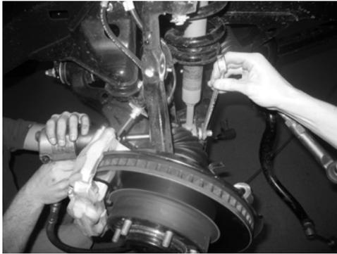
9. Remove the strut assembly from the vehicle and mount it in a bench vise. Install the Hell Bent Steel Strut extension on the top of the strut, hold the part up to start the factory nuts onto the factory studs.
