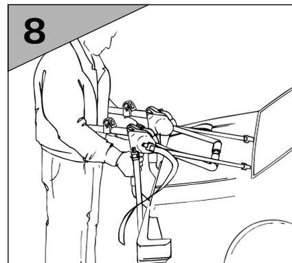
Tighten top straps so that the Voyager stays in position and the bike arms are pointing slightly upwards. On 3 bike carrier attach side strap to side seam of trunk hatch or door.
