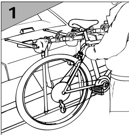
Place first bike onto Voyager. Position the inside pedal so that it doesn't come in contact with the vehicle.
