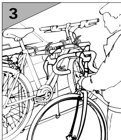
Mount second bike in the opposite direction. The second bike should be secured to the first bike using strap or rope.
