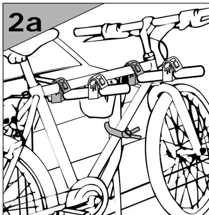
Using straps or rope (not supplied), secure the bike to the lower arms of the Voyager.
