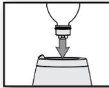
Failure to ensure the tank is seated correctly could cause the unit to leak water from the tank.
