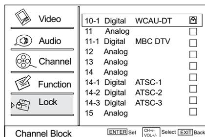
Press **CH+/-** button to select the channel you want to lock, then press **ENTER** button to confirm. The channel is locked and a lock mark appears in the pane. If you want to unlock the channel, repeat the operation above again. Then press **EXIT** to exit step by step.
