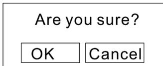
Press **VOL+/-** button to select OK or Cancel, then press **OK** to confirm. If **OK** the parameter will return to the factory set.
