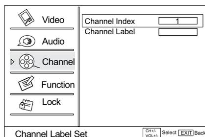
Then press **CH+/-** button to select Channel Index and **VOL+/-** button to select the position of the item that you want to change, afterward press **INPUT** to input the numbers and symbols and **ENTER** button to confirm.
