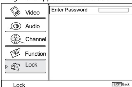
❷ Press **VOL+ / ENTER** button to enter and then press digits button to input the digits (The initial password is 0000. If you forget your password, you can always input 9443 to regain control). The menu will display as follows:
