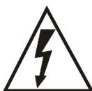
The lightning flash with arrowhead symbol, within an equilateral triangle is intended to alert the user to the presence of uninsulated dangerous voltage within the product's enclosure that may be of sufficient magnitude to constitute a risk of electric shock.
