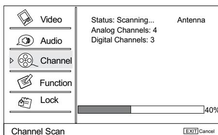
All channels now available will be automatically preset in order. After the search has finished, the first program number will display on the screen. This search automatically adds only the active channels in your area to the TV's memory. It deletes any channels on which there is no broadcast or a poor signal. The channels found are automatically saved.
