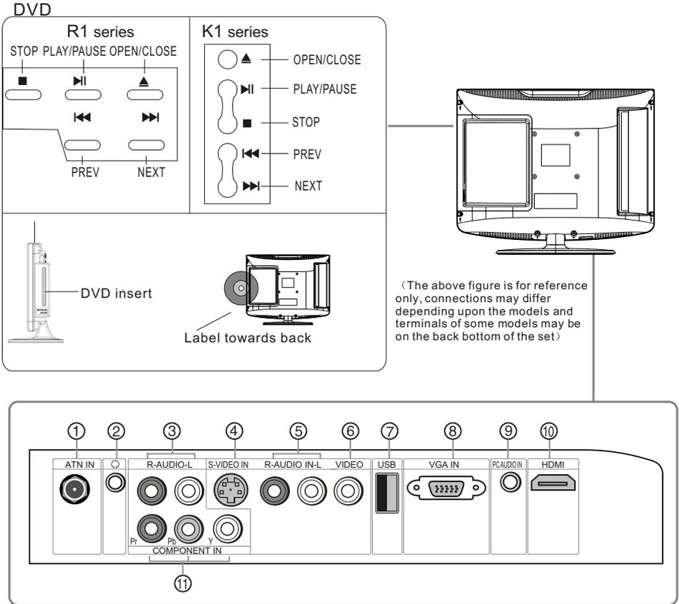
1. **ANT IN (Antenna Input)** Connect cable or antenna signals to the TV, either directly or through your cable box.
