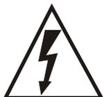
The lightning flash with arrowhead symbol, within an equilateral triangle is intended to alert the user to the presence of uninsulated dangerous voltage within the product's enclosure that may be of sufficient magnitude to constitute a risk of electric shock.
