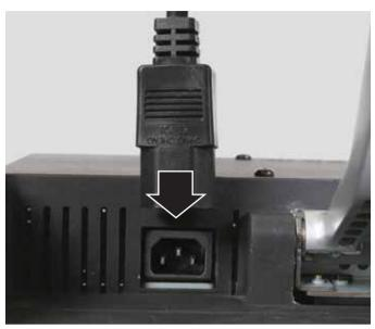
2 Plug the power cord into a correctly grounded power outlet. We recommend using a surge protector to protect your monitor from voltage spikes.
