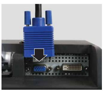
3 Make sure that your computer is turned off, then connect the other end of the video cable to the matching video port on the back of your computer.
