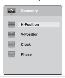
**H-Position**—Moves the display image left and right. You can also press the **Auto** button to configure the horizontal position automatically. **V-Position**—Moves the display image up and down. You
