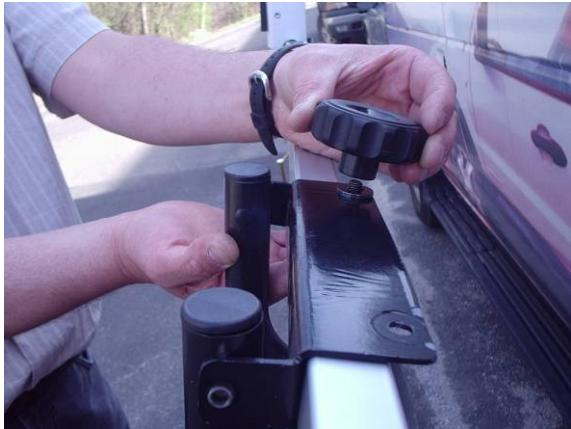
Position handle assembly (F) over lower handle tube. Attach using M8x40mm carriage bolts (M), washers (H), and knobs (L) as shown.
