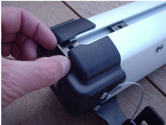
Insert two square nuts (I) in top slot of arm and slide to opposite end.
