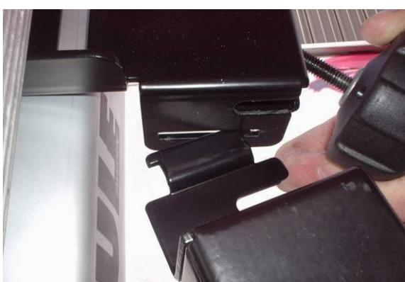
Insert bottom clamp (U) into ladder bracket assembly (N) as shown.
