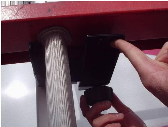
Close bottom clamp (U) and rotate knob into slot in bottom clamp.
