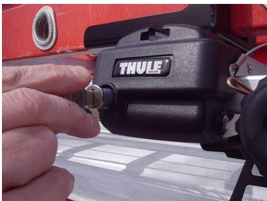
Insert lock cylinder into endcap using square headed key.
