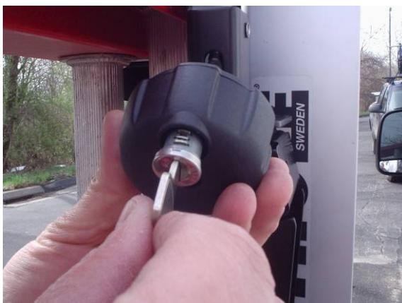
Insert lock cylinder (X) into knob using square headed key (Y).
