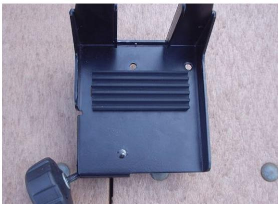
Insert rubber pad (T) into ladder bracket assembly (N).
