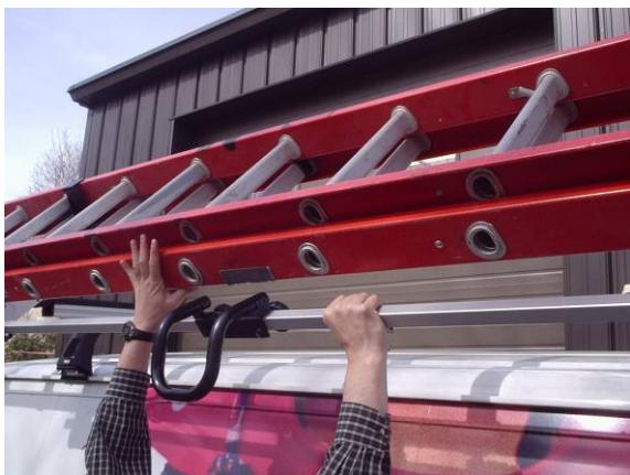
Rotate ladder system down onto bar mounts.
