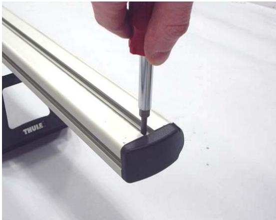
Remove end cap from one side of load bars.
