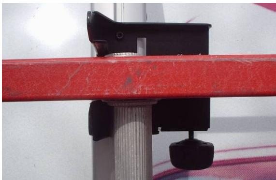
Lift ladder and place into ladder bracket assemblies.
