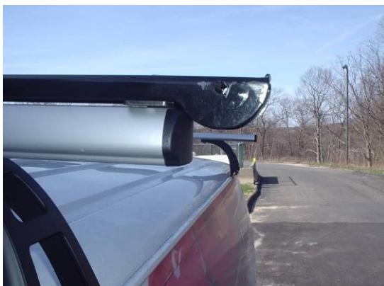
Place bar mount (A) on load bar as shown.
