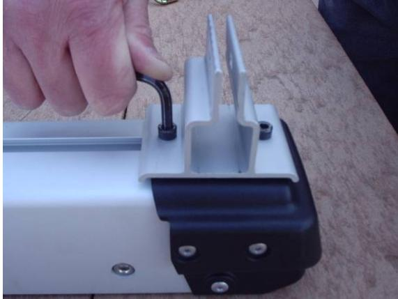
Position tube holder (E) as shown and attach to square nuts in arm using M6x12mm allen bolt (J). Loosely assemble carriage bolt M8x25mm (G), washer (H) and knob (L) to tube holder (E).
