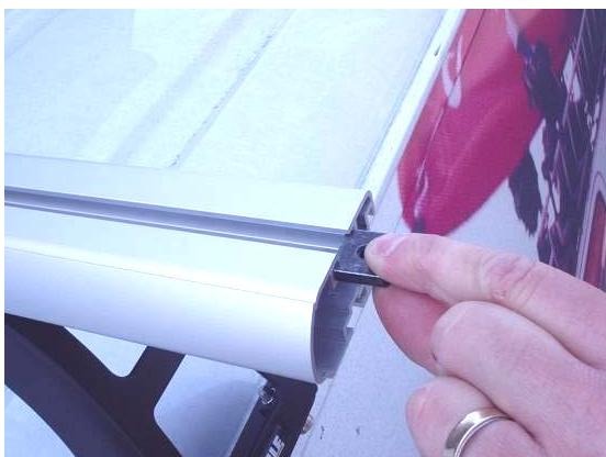
Insert two square nuts (I) in top slot of load bar.
