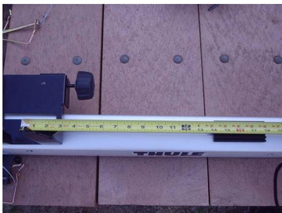
Move rubber pads (T) same distance apart from ladder bracket as ladder width.
