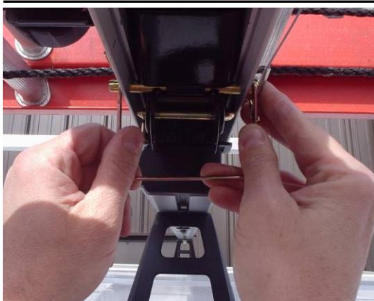
With arm latched, install pin with lanyard through hole in arm and place safety clip on end of pin.
