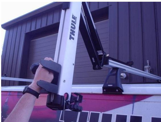
Pull arm out and down to lower to side of vehicle.
