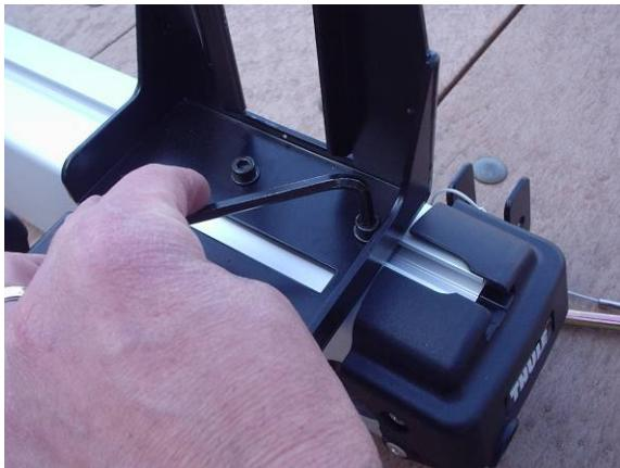
For one arm, position ladder bracket (N) against end cap as shown.
