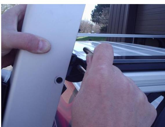
Place arm assembly (B) vertically onto bar mount (A).
