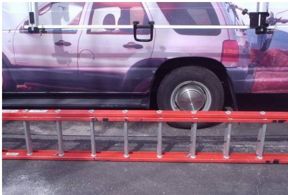
Center ladder under lift system prior to loading.
