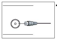
Connect an antenna cable to the antenna connection of the plasma TV and to the TV antenna socket.
