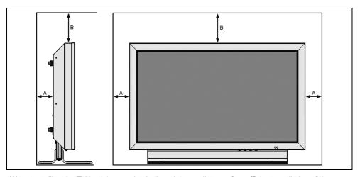
When installing the TV in niches, maintain the minimum distance for sufficient ventilation of the device: 10 cm from the side and back, 20 cm from the top.
