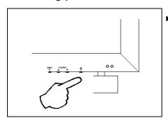
Press the Standby button at the right on the underside of the plasma TV.
