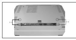
► Remove the four screws (1) that secure the foot to the device.
