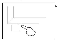
Press the ON/OFF switch at the left on the back of the plasma TV.
