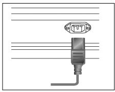
Plug the power cable supplied into the power connector of the plasma TV.
