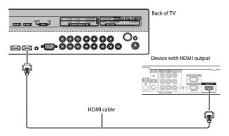
3 Connect the other end of the cable to the HDMI1 or HDMI2 jack on the back of your TV or the HDMI3 jack on the side of your TV.
