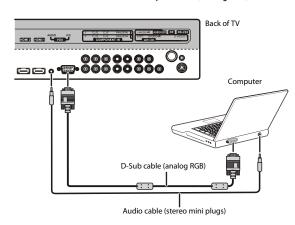
3 Connect an audio cable to the AUDIO OUT jack on the computer, then connect the other end of the cable to the VGA AUDIO jack on the back of your TV.
