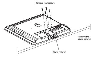
2 Remove the four screws holding the stand column to your TV, then remove the stand column.
