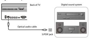
3 Connect the other end of the cable to the **DIGITAL OUTPUT** jack on the back of your TV.
