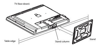
3 Align the holes in the stand with the holes in the stand column. Secure the stand to the column with four M5 screws (37" model) or five M5 screws (42" model) provided.
