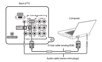
3 Connect an audio cable to the AUDIO OUT jack on the computer, then connect the other end of the cable to the VGA IN AUDIO jack on the back of your TV.
