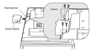
**4** With the wider side of the stand facing down, align the tabs on the stand column with the holes on the stand, then gently push the stand toward the stand column until it clicks into place.
