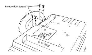
2 Remove the four screws holding the stand column to your TV, then remove the stand and the stand column.
