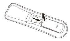
Insert two AAA batteries into the battery compartment. Make sure that the + and - symbols on the batteries match the + and - symbols in the battery compartment.
