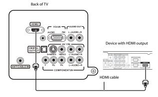
3 Connect the other end of the cable to the HDMI1 or HDMI2 jack on the back of your TV.
