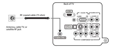
2 Connect the other end of the cable to the ANT/CABLE IN jack on the back of your TV.
