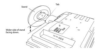
**5** Secure the stand with the four stand screws.
