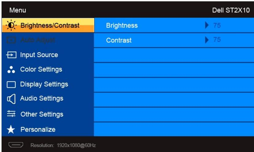
**NOTE:** Auto Adjust is only available when you are using the analog (VGA) connector.
