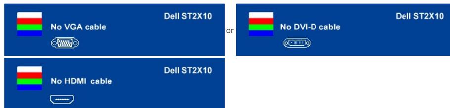
4. This box also appears during normal system operation, if the video cable becomes disconnected or damaged.
