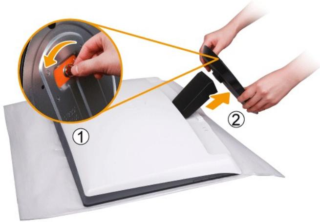
After placing the monitor panel on a soft cloth or cushion, complete the following steps to remove the base.
