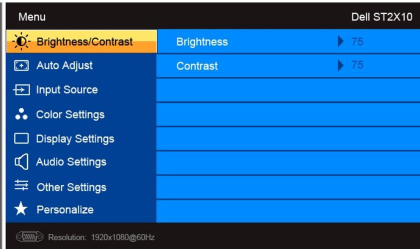
**Brightness** Brightness adjusts the luminance of the backlight.
