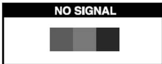
No Signal screen is displayed when the D-Sub signal connector is connected but the status of the LCD TV is on DPMS mode.
