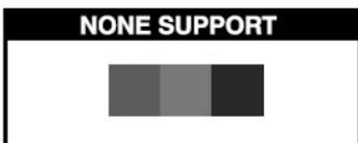
None support screen is displayed when the applied frequency is under or over factory preset timings.
