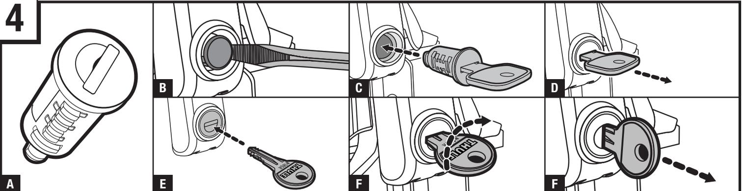
**Thule strongly recommends the use of locks to deter theft. As shown, follow these easy steps for installing the lock cylinders.**
