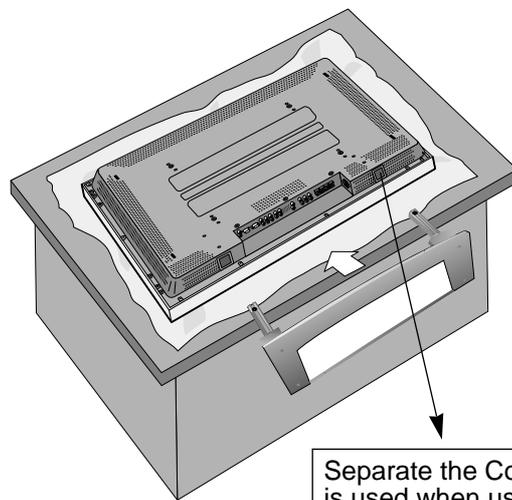
Separate the Cover Stand. (It is used when using for wall mounting, so store it.)
