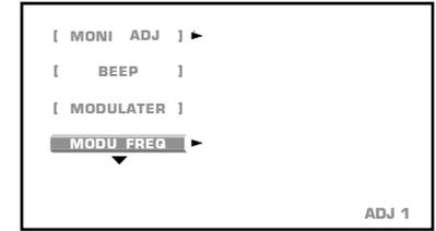
2. Press the [▶] button to display the frequency setting screen.
