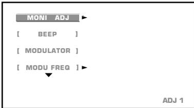
2. Press the [▲] or [▼] button to select the desired adjustment menu.
