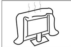
Do not block the ventilation holes in the back cover. Adequate ventilation is essential to prevent failure of electrical components.
