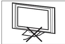
Do not trap the power supply cord under the television receiver.
