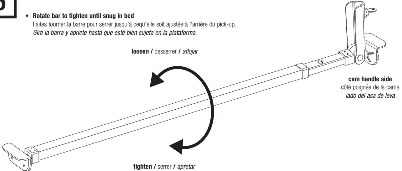
**Over tightening can cause damage to truck bed. Do not over tighten before closing cam handle.**
