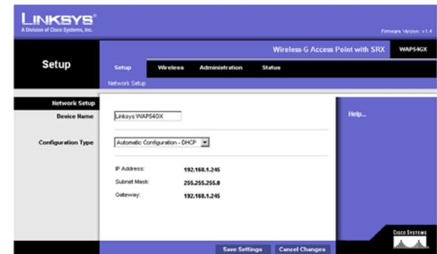
Figure 6-2: Setup - Automatic Configuration - DHCP Screen
