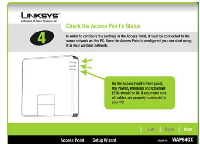
Figure 5-5: Check the Access Point's Status Screen
