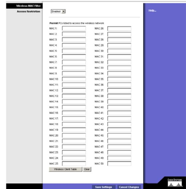
Figure 6-11: Wireless - Wireless MAC Filter Screen
