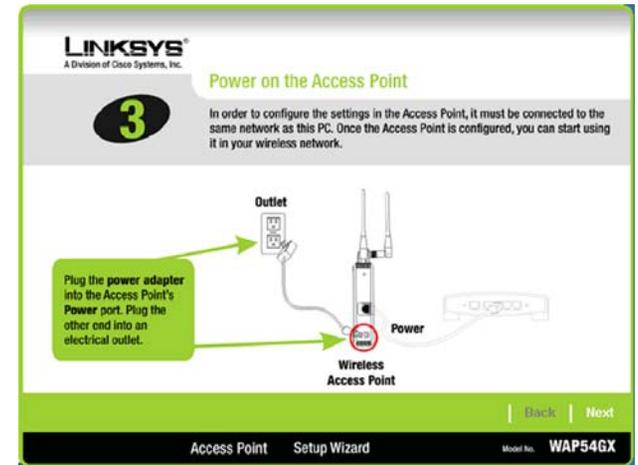
Figure 5-4: Power on the Access Point Screen
