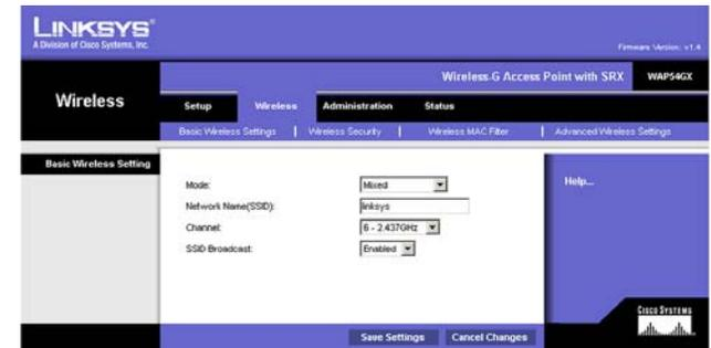
Figure 6-4: Wireless - Basic Wireless Settings Screen
