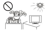
The vents and other openings in the cabinet are designed for ventilation. Do not cover or block these vents and openings since insufficient ventilation can cause overheating and/or shorten the life of the product.
