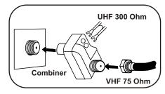
Connect the 75 Ohm cable from combination VHF/UHF antenna to the antenna jack.
