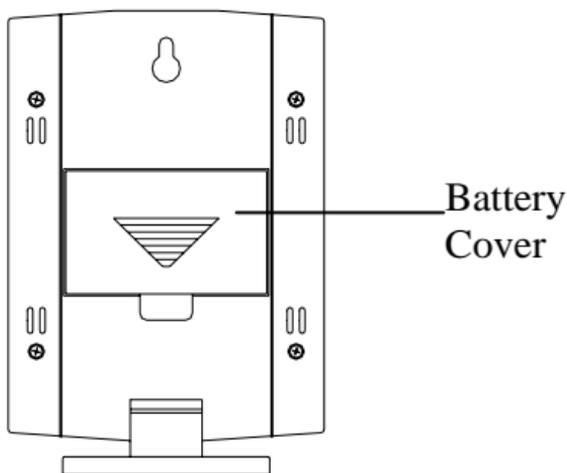
2. Observing the correct polarity, install 2 AA batteries.
