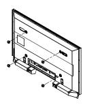
4 Remove the Safety Pins. Fasten the 4 plastic latches assembled at step (③) on the back side of the PDP using the guide holes of the wall mount, push (①) and hook (②) down to secure the PDP on the wall mount as illustrated. Secure the PDP by inserting the Safety Pins, not to fall from the wall mount.
