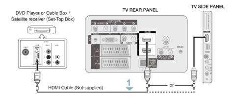
1. Connect an HDMI Cable(Not supplied) between the HDMI IN (1, 2 or 3) jack on the TV and the HDMI jack on the Cable Box/Satellite receiver (Set-Top Box).
