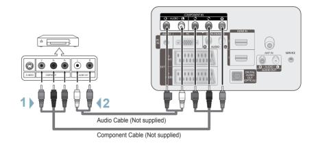
Connect a Component Cable(Not supplied) between the COMPONENT IN [Y, PB, PR] jacks on the TV and the COMPONENT jacks on the Cable Box/Satellite receiver (Set-Top Box).
