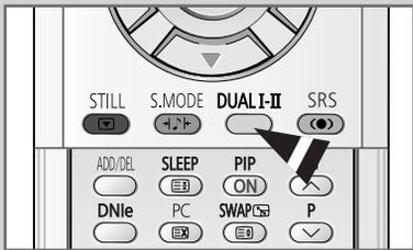
The "DUAL I-II" button displays/controls the processing and output of the audio signal. When power is switched on, the mode is automatically preset to either "Dual I" or "Stereo", depending on the current transmission.
