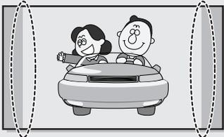
Although digital broadcasting must be in the wide screen (16:9) HD format, broadcasters sometimes show programs made originally in the regular screen format (4:3) by converting the signals into digital form, in which case the left and right side edges of the screen are cropped.
