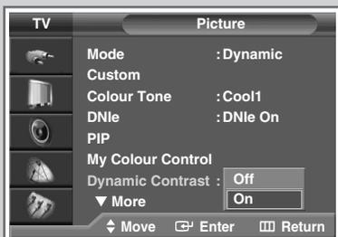
*Dynamic Contrast automatically detects the visual signal and adjusts to create optimum contrast.*
