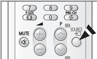
*Use the remote control to switch between viewing signals from connected equipment, such as VCR, DVD, Set-Top Box, and the TV source (broadcast or cable).*
