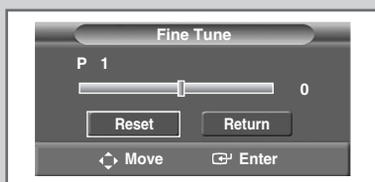
*If the reception is clear, you do not have to fine tune the channel, as this is done automatically during the search and store operation. If the signal is weak or distorted, you may have to fine tune the channel manually.*
