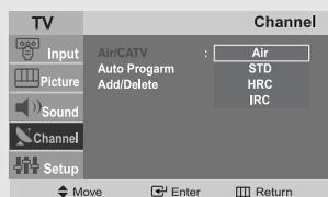
Note : STD, HRC and IRC identify various types of cable TV systems. Contact your local cable company to identify the type of cable system that exists in your particular area.
