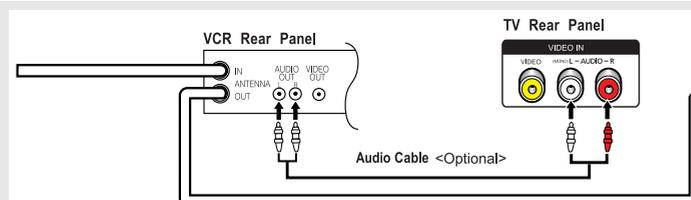
If you have a “mono” (non-stereo) VCR, use the Y-connector (not supplied) to hook up to the left and right audio input jacks of the TV.
