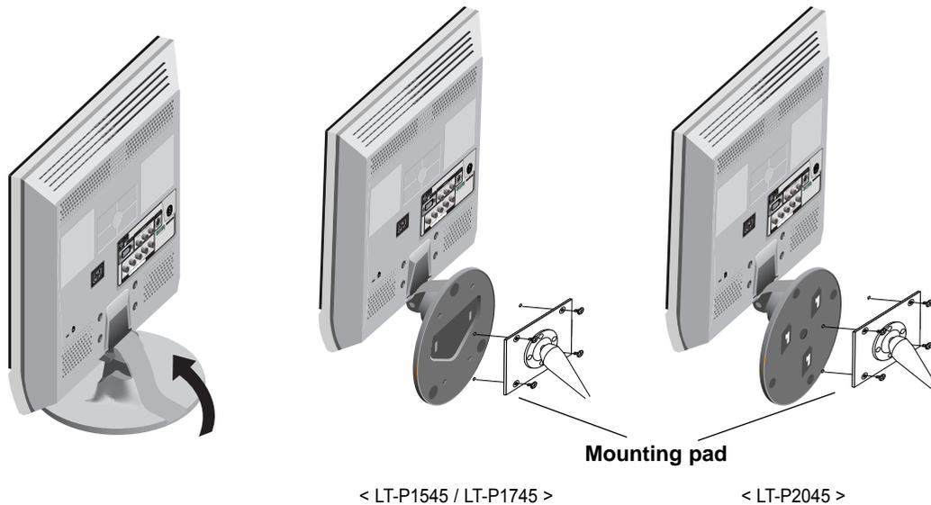
Align the mounting interface pad with the holes in the rear cover mounting pad and secure it with the four screws that come with the arm-type base, wall mount hanger or other bases.
