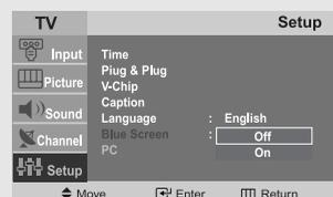
◀ Pressing the **UP/DOWN ▲▼** buttons will alternate between “On” and “Off”.
