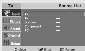
Note: You can also press the **SOURCE** button on the remote to choose the Input source.
