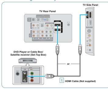
Connect an HDMI Cable between the HDMI IN (1, 2 or 3) jack on the TV and the HDMI jack on the DVD Player or Cable Box/Satellite receiver (Set-Top Box).
