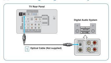
Connect an Optical Cable between the "DIGITAL AUDIO OUT (OPTICAL)" jacks on the TV and the Digital Audio Input jacks on the Digital Audio System.
