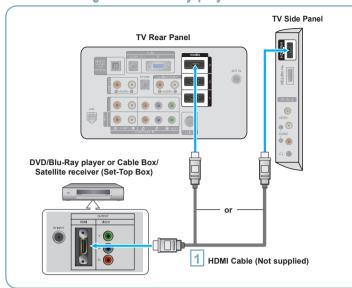
Connect an HDMI Cable between the HDMI IN (1, 2, 3 or 4) jack on the TV and the HDMI jack on the DVD/Blu-Ray player or Cable Box/Satellite receiver (Set-Top Box).
