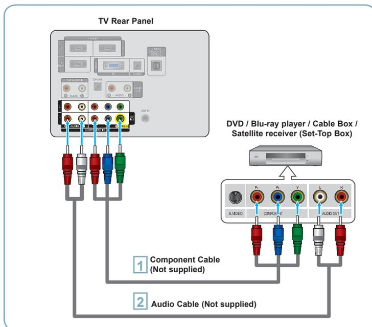
**1** Connect a Component Cable between the COMPONENT IN (1 or 2) [Y, Pb, Pr] jacks on the TV and the COMPONENT [Y, Pb, Pr] jacks on the DVD / Blu-ray player / Cable Box / Satellite receiver (Set-Top Box).
