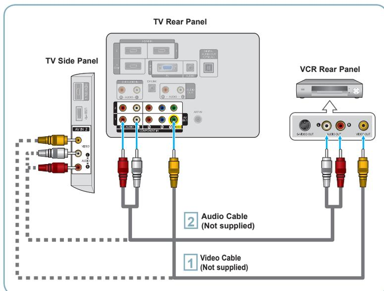
**1** Connect a Video Cable between the AV IN 1 [Y/VIDEO] or AV IN 2 [VIDEO] jack on the TV and the VIDEO OUT jack on the VCR.
