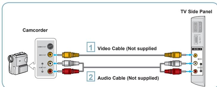
**1** Connect a Video Cable between the AV IN 2 [VIDEO] jack on the TV and the VIDEO OUT jack on the camcorder.
