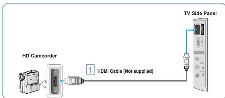
**1** Connect an HDMI Cable between the HDMI 4 jack on the TV and the HDMI OUT jack on the camcorder.
