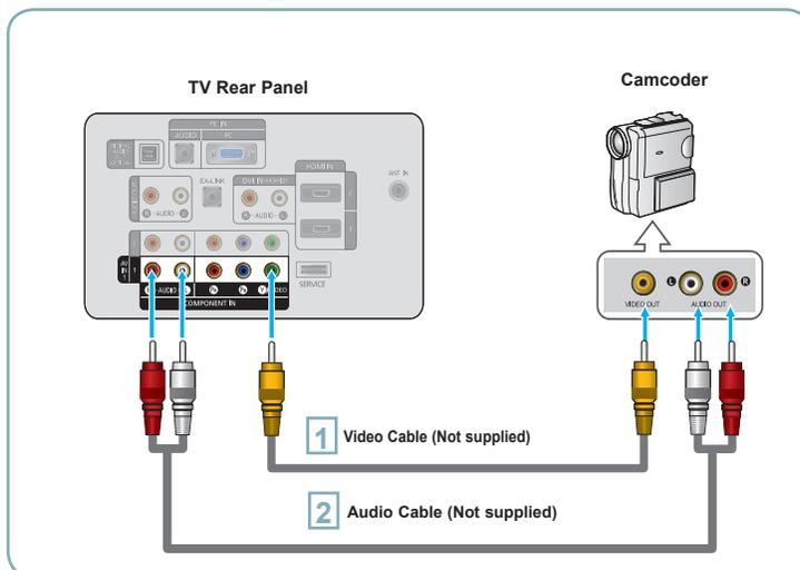
**1** Connect a Video Cable between the AV IN 1 [Y/VIDEO] jack on the TV and the VIDEO OUT jack on the camcorder.
