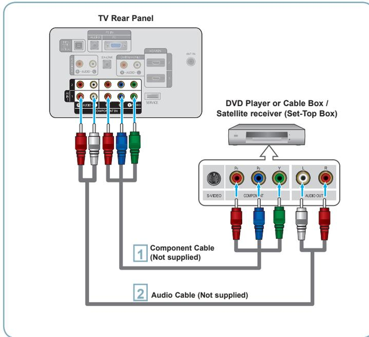
**1** Connect a Component Cable between the COMPONENT IN (1 or 2) [Y, Pb, Pr] jacks on the TV and the COMPONENT [Y, Pb, Pr] jacks on the DVD Player or Cable Box/Satellite receiver (Set-Top Box).
