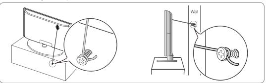
4. Verify all connections are properly secured. Periodically check the connections for any sign of fatigue or failure. If you have any doubt about the security of your connections, contact a professional installer.
