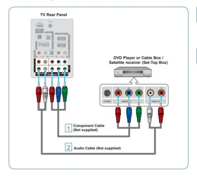
Connect a Component Cable between the COMPONENT IN (1 or 2) [Y, PB, PR] jacks on the TV and the COMPONENT [Y, PB, PR] jacks on the DVD Player or Cable Box/Satellite receiver (Set-Top Box).
