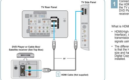
Connect an HDMI Cable between the HDMI IN (1, 2 or 3) jack on the TV and the HDMI jack on the DVD Player or Cable Box/Satellite receiver (Set-Top Box).
