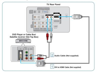
Connect a DVI to HDMI Cable or DVI-HDMI Adapter between the HDMI IN 2 jack on the TV and the DVI jack on the DVD Player or Cable Box/ Satellite receiver (Set-Top Box).
