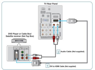
Connect a DVI to HDMI Cable or DVI-HDMI Adapter between the HDMI IN 1 jack on the TV and the DVI jack on the DVD Player or Cable Box/ Satellite receiver (Set-Top Box).
