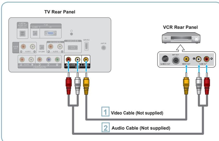
**1** Connect a Video Cable between the AV IN [VIDEO] jack on the TV and the VIDEO OUT jack on the VCR.
