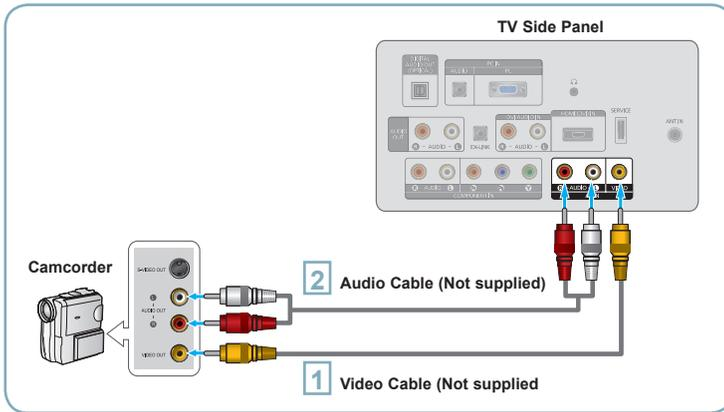
**1** Connect a Video Cable between the AV IN [VIDEO] jack on the TV and the VIDEO OUT jack on the camcorder.
