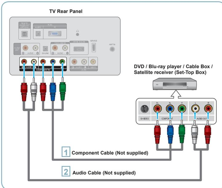
**1** Connect a Component Cable between the COMPONENT IN [Y, P<sub>B</sub>, P<sub>R</sub>] jacks on the TV and the COMPONENT [Y, P<sub>B</sub>, P<sub>R</sub>] jacks on the DVD / Blu-ray player / Cable Box / Satellite receiver (Set-Top Box).
