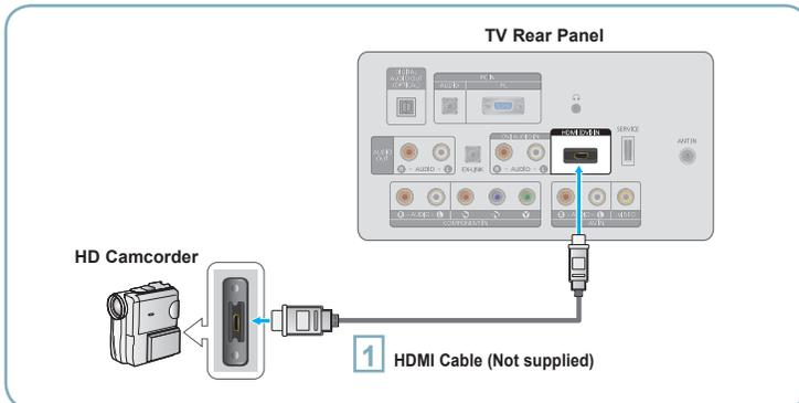
**1** Connect an HDMI Cable between the HDMI (DVI) IN jack on the TV and the HDMI OUT jack on the camcorder.
