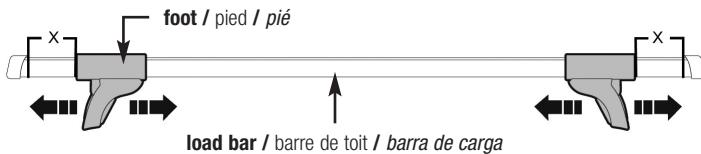
**NOTE:** The best way to make sure your bars are centered is to measure how much bar sticks out from the outside of the foot (X) and then to adjust the bar until those measurements are equal.
