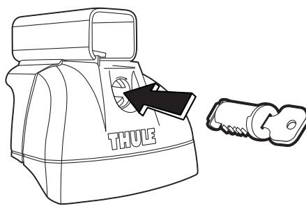
**b. Insert cylinder into foot.**
