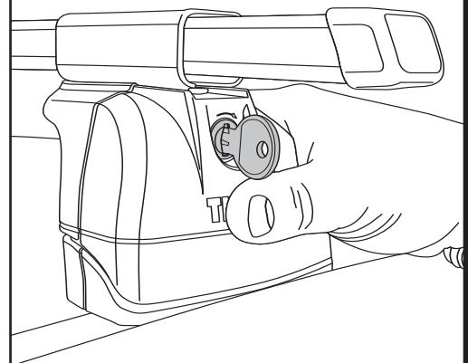
**c. Once you have installed the lock core, insert the "N" series key. Press thumb against Thule logo and hold. This will prevent the cover from "popping" when turning the key clockwise to the locked position.**
