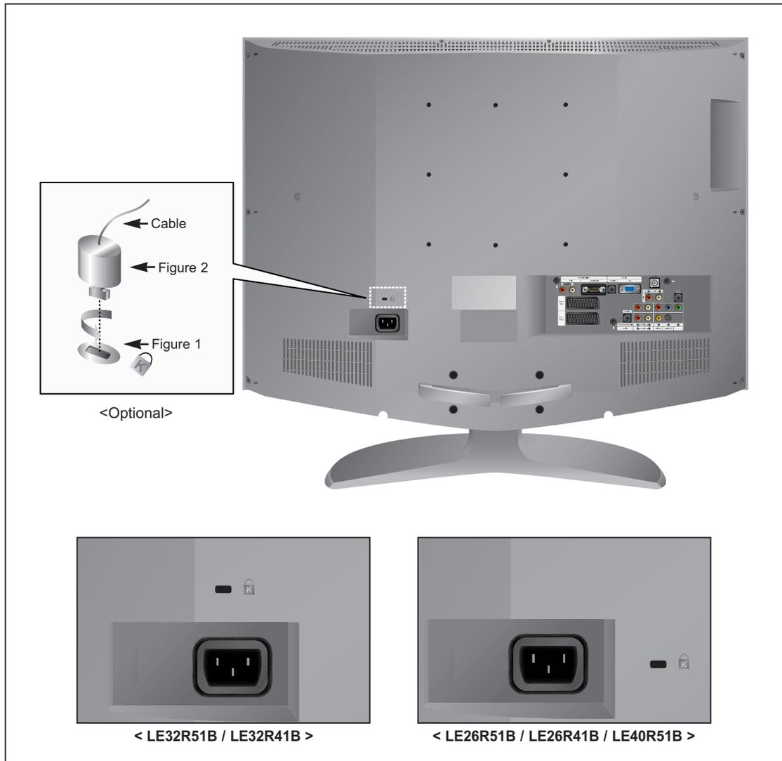
1. Insert the locking device into the Kensington slot on the LCD TV (Figure 1), and turn it in the locking direction (Figure 2).
