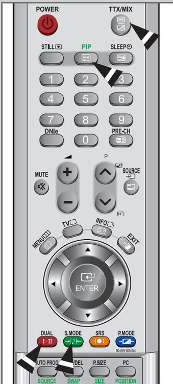
*The various topics included in the teletext pages are colour-coded, and can be selected by pressing the coloured buttons on the remote control.*
