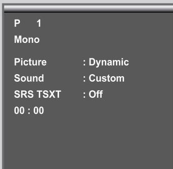
*You can set the TV's clock so that the current time is displayed when you press the **INFO** button. You must also set the time if you wish to use the automatic On/Off timers.*
