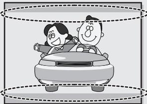
Although digital broadcasting must be in the wide screen (16:9) HD format, broadcasters sometimes show programs made originally in the regular screen format (4:3) by converting the signals into digital form, in which case the left and right side edges of the screen are cropped.
