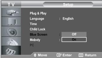
*If no signal is being received or the signal is very weak, a blue screen automatically replaces the noisy picture background.
