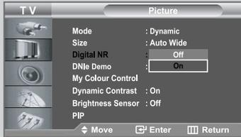
*If the signal received by your television is weak, you can activate this feature to help reduce any static and ghosting that may appear on the screen.*
