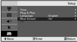
*If no signal is being received or the signal is very weak, a blue screen automatically replaces the noisy picture background. If you wish to continue viewing the poor picture, you must set the "Blue Screen" mode to "Off".*
