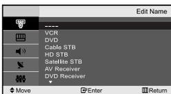
*Name the device connected to the input jacks to make your input source selection easier.*
