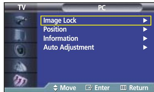
3 Press the ▲ or ▼ button to select "Auto Adjustment", then press the ENTER button. The message "Auto Adjustment in progress." appears on the screen and the picture adjustments are automatically activated.
