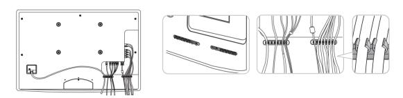
Do not pull the cables too hard when arranging them. This may cause damage to the product's connection terminals.
