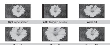
Screen Fit displays the full image without any cut-off when HDMI (720p / 1080i / 1080p) or Component (1080i / 1080p) signals are inputted.
