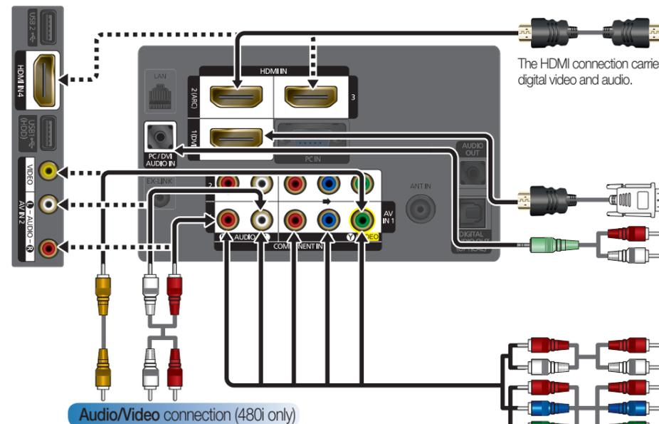
When connecting to AV IN 1 on the back of your TV, attach the video cable (yellow) to the green jack next to the AV IN 1 label. The jack will not match the color of the video cable (yellow).
