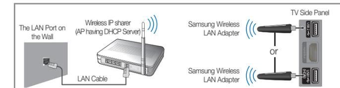
Samsung's Wireless LAN adapter supports the IEEE 802.11A, IEEE 802.11B, IEEE 802.11G, and IEEE 802.11N wireless communication protocols. For your TV to connect to your network, the wireless router or modem you use must also support one of these protocols. The fastest of these protocols is IEEE 802.11N.
