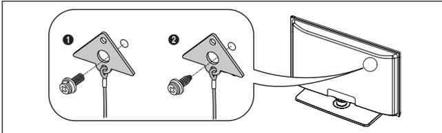
2. Firmly fasten the screw you provided (size M4xL20 or similar) to the wall or cabinet where the TV is to be installed.
