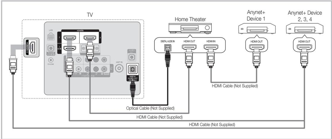
1. Connect the **HDMI IN (1(DVI), 2, 3 or 4)** jack on the TV and the **HDMI OUT** jack of the corresponding Anynet+ device using an HDMI cable.
