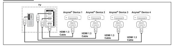
Connect the [HDMI 1], [HDMI 2], [HDMI 3] or [HDMI 4] jack on the TV and the HDMI OUT jack of the corresponding Anynet<sup>+</sup> device using an HDMI cable.
