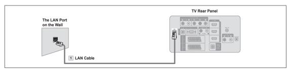
1. Connect the [LAN] port on the rear panel of the TV and the LAN port on the wall using the LAN cable.
