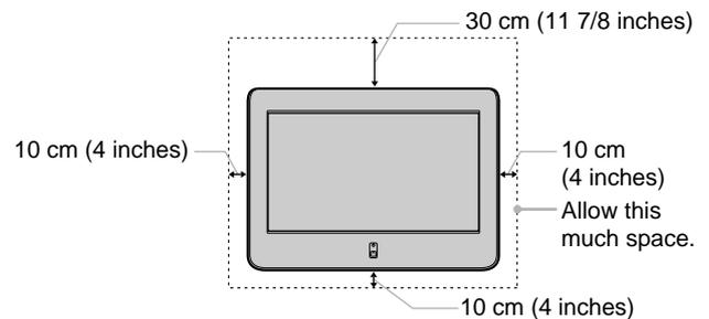
When installing the unit using a stand
