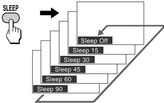
While the Sleep timer is activated, the ⏰ (Timer) LED on the TV lights up in red.
