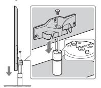
**2** Attach the TV and Table-Top Stand with the supplied screw and hexagon wrench.
