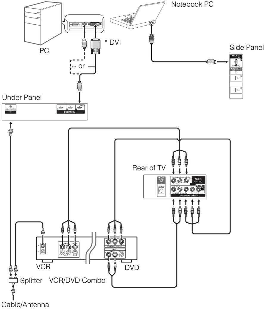
\* DVI does not support audio signals. Connect the audio output of the PC to the PC speakers or an A/V receiver to listen to sound from the PC.
