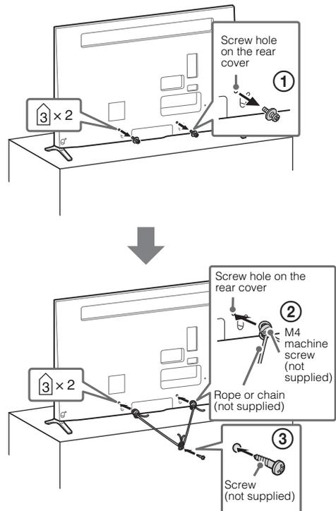
The length of the M4 machine screw differs depending on the rope or chain diameter. Please see below illustration.
