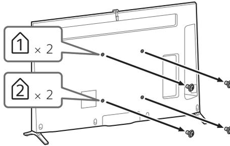
**2** Before installing the Wall-Mount Bracket, attach the Wall-Mount Attachment (supplied with the TV) to the rear of the TV (to make it parallel with the wall).
